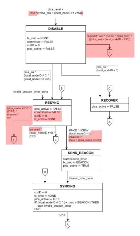
Figure 148-3--PLCA Control state diagram, part a
