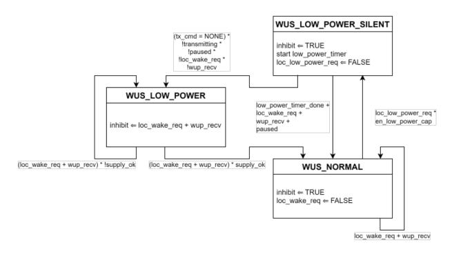
Figure 8-2--PHY power mode state diagram
