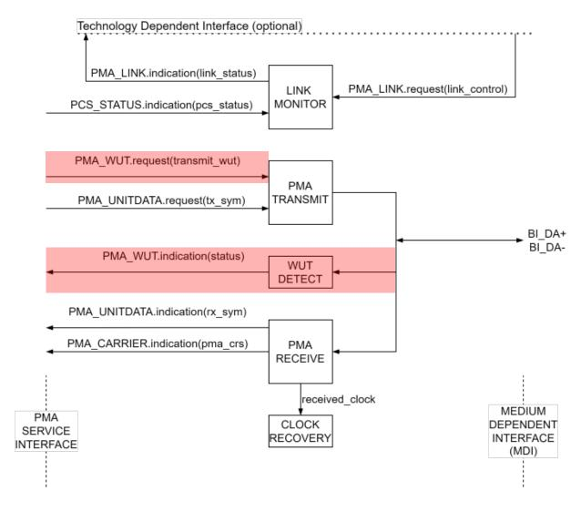
Figure 147-12--PMA functional block diagram
