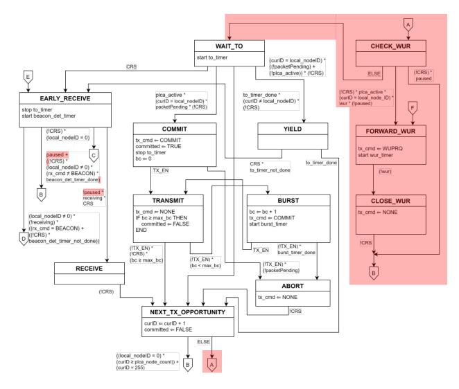
Figure 148-4--PLCA Control state diagram, part b
