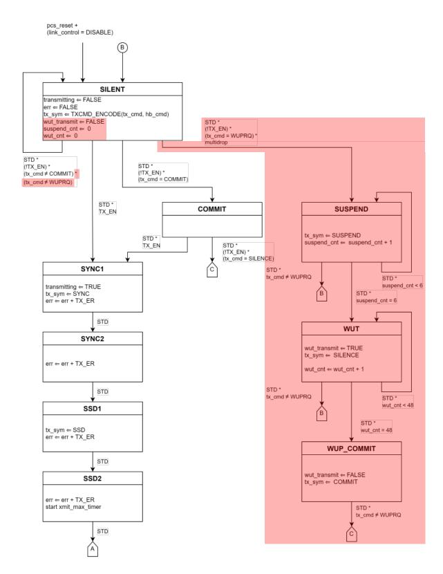
Figure 147-4--PCS Transmit state diagram, part a
