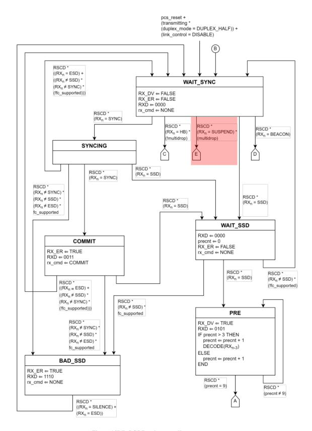
Figure 147-7--PCS Receive state diagram, part a
