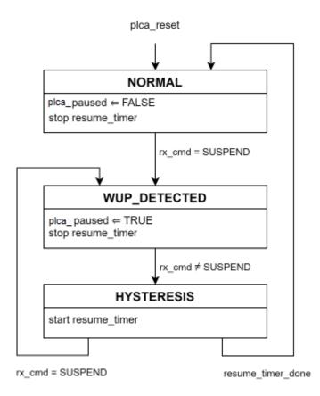
Figure 148-8--PLCA Pause state diagram
