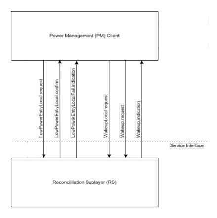
Figure 8-1--PM Client and RS interlayer service interfaces
