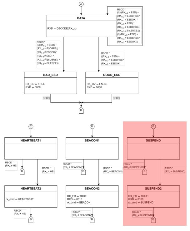
Figure 147-8--PCS Receive state diagram, part b
